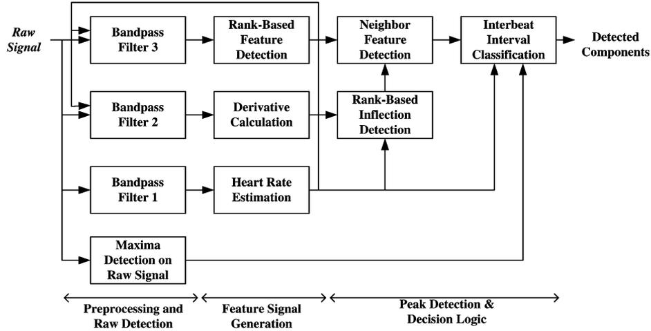
Fig. 4. Block diagram showing the architecture and individual stages of the new detection algorithm for peak component detection in pressure signals.
