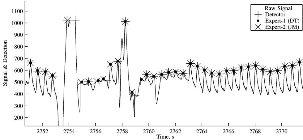
Fig. 8. Example showing a SpO<sub>2</sub> signal and the systolic peak (SBP) identified by the two experts and the detection algorithm. In this case the experts and algorithm labeled different peaks in the regions of artifact. Clearly Expert-1 (DT) made the correct choice and Expert-2 (JM) needs more training.
